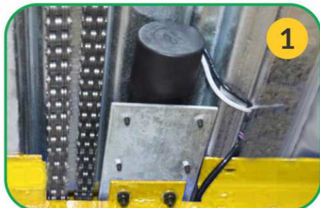
1. Special electromagnet feedback for car garage (Fig. 01).
